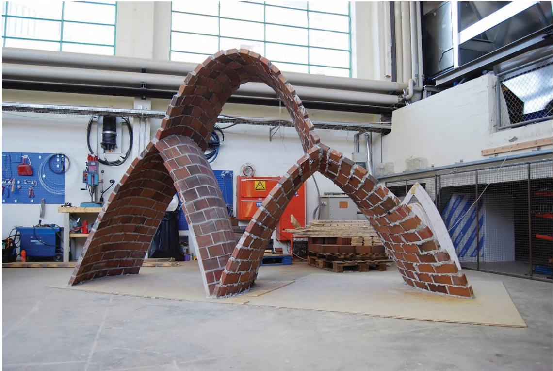
Figure 6 Nested Catenaries , conducted by Defne Sunguroğlu Hensel, engineer Guillem Baraut Bover and master mason Øyvind Buset, Oslo, 2012 [Phase 2]: A Cavity Wall. The design involved the use of three shells; two of which could be articulated independently while remaining in relation to the third shell above. These are catenary shells with synclastic and anticlastic surface curvatures connected with the shell above, which displays a transition from a concave to convex transverse section. The reason for two different base-shell solutions was to study their implications on construction and structural behaviour under non-uniform loads.
